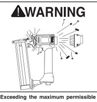
Exceeding the maximum permissible operating pressure may damage the nailer and cause it to malfunction. To protect yourself from personal injury, DO NOT allow the air pressure to exceed the recommended pressure for this nailer!
